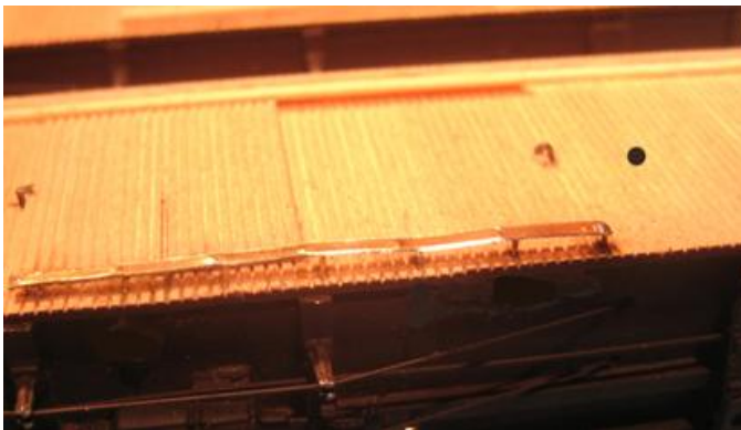
Fig. 4 and 5. Close-up shots of the brass strips soldered to the wire standoffs.
