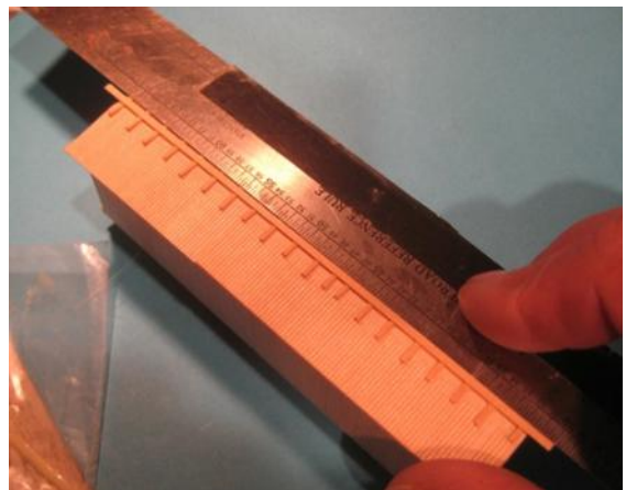
Fig. 8. Take a straight edge and make sure it is absolutely straight.
