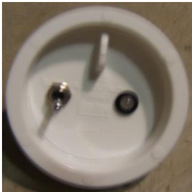
Left. Manual Tortoise Control with DPDT toggle switch with red/green 2-lead 5mm LED with holder. Right. DCC Tortoise Control with normally-open push-button switch with red/green 2-lead 5 mm LED with holder.
