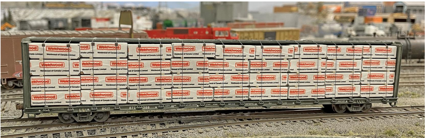
Photo 7. BCIT lumber car. No load on model as bought. Each block of 4x8s was individually wrapped (note wrinkles in wrappers), and stacked with wood strips between blocks. Note ties holding the blocks on, with black reinforcements at the top to prevent damage to the edges of the 4x8s.
