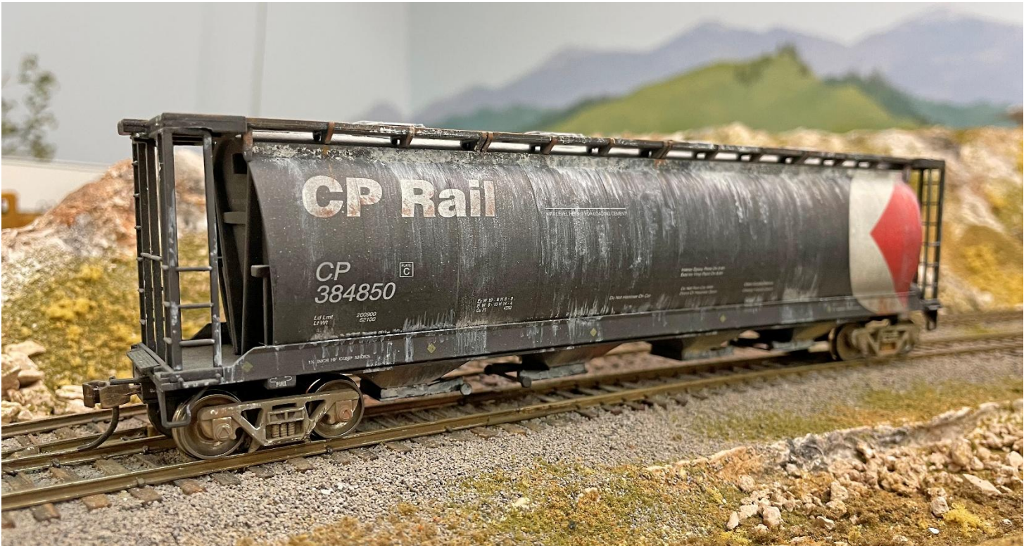
Photo 6. CP cylindrical hopper, used for cement transport. Prototype photographed at Exshaw. Weathering of model consists of a) overall fading of the black plastic car sides, and b) cement streaks as on the prototype, using a fine paintbrush and cosmetic sponge.
