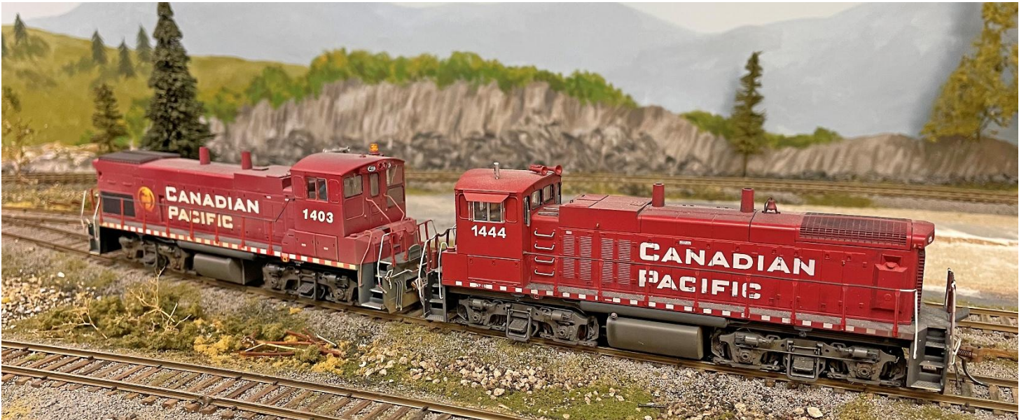
Photo 4. MP15 switchers. In the prototype, 1403 is the AC version, 1444 is DC.
