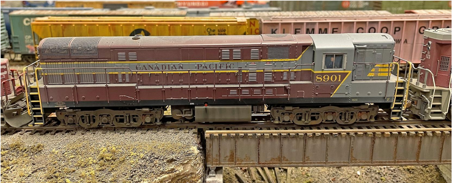
Photo 2. Trainmaster H-24-66. Lightly weathered overall, but trucks weathered to show detail in side frames.
