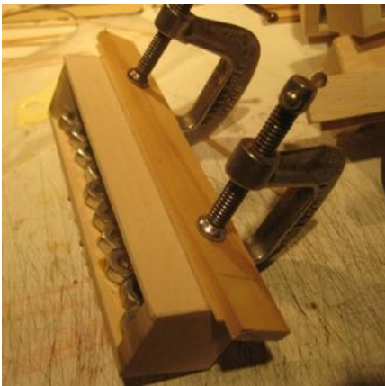
Figs. 13 and 14. Although it is hard to see, there is a half inch wide strip of wood that distributes the pressure of the clamps and is positioned so as to allow the pencil line guide to remain visible. Note that Fig 13 shows some of the weights I added.
