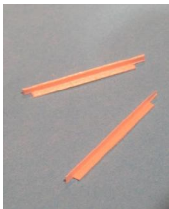
Fig. 27. End beams are formed from angle stripwood.
