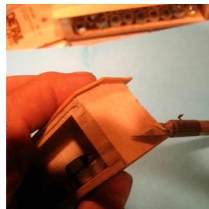
Figs. 18. and 19. Look out!! This is asking for trouble. Be sure you know how the wood grain is running to avoid the blade being drawn into the scribed end.
