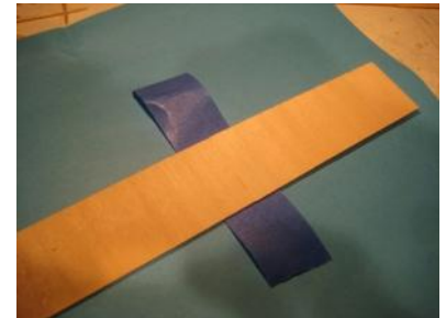
Fig. 3. Place two scribed panels together end-to-end, scribed sides down, on a piece of painter's tape.
