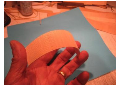
Fig. 6. After the glue has dried, carefully flex the panel to ensure the joint is solid and will not fail.
