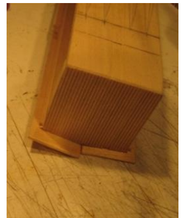
Fig. 15. Here is a view of the underside of the overhang with the clamps removed.
