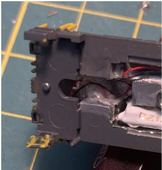
Fig. 6. Metal end-piece with nano LED glued in for head light and tail light.
