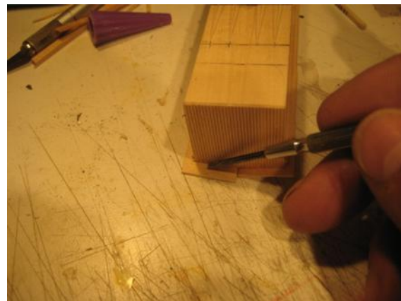
Fig. 17. Spread out the bead of super glue using a sharp square-edged screwdriver.
