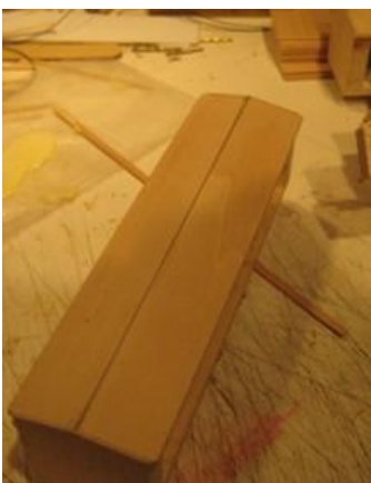
Fig. 12. Pencil line down the roof centerline to guide gluing roof sheathing.
