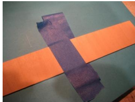
Fig. 5. After applying glue sparingly to the edges, lay the panels flat again and tape down with a second piece of tape, allowing the lengthened panel to dry overnight.
