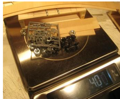
Fig. 10. A million years ago, I obtained two boxes of 1000 1/4-20 and 1/4-28 nuts. I will NEVER use that many, so they go in for weights. I glue them in with contact cement and spread the weight out both width- and lengthwise.
