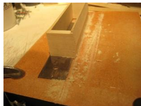
Fig. 11 Sanding down excess roof overhang using an old Athearn steel weight as a guide.
