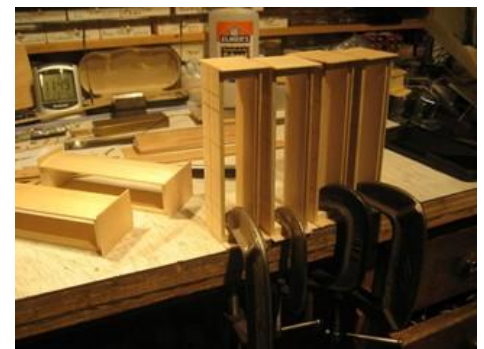
Fig. 7. Batch gluing scribed ends to the core boxes assembled in Part 1.
