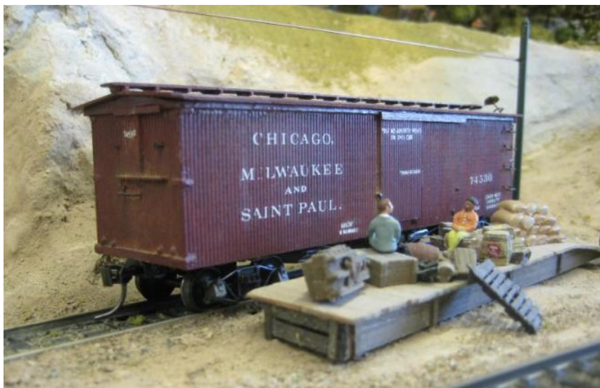
Fig. 12. Note the NBWs on the lower part of this boxcar's end siding that represent the connection point of the longitudinal truss rods.
