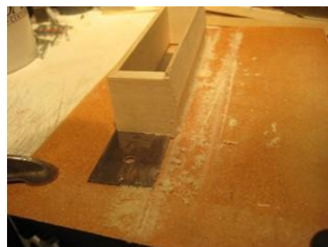
Fig. 17. Sanding down excess roof overhang using an old Athearn steel weight as a guide.
