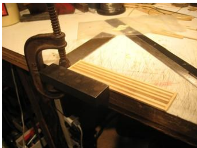
Fig. 3. I use a machinist's square clamped to the edge of my bench to get everything square.
