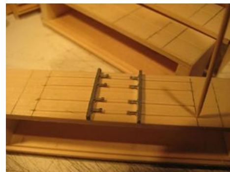
Fig. 18. Queen posts are laying flat while the monofilament string is tightened. Note the toothpick inserted into the last hole to hold the string tight while knotting and gluing the end.
