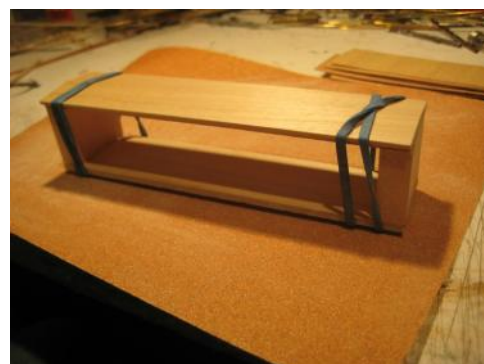
Fig. 13. Assembling the basic box core by gluing the ends and roof to the floor.
