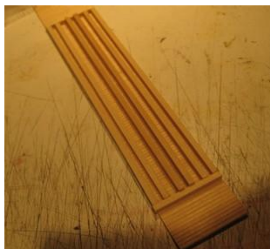
Fig. 4. Here are the center sills, stringers, side sills, and end sills laid out on top of the floor made from scribed wood siding. The floor has not been cut to length yet.
