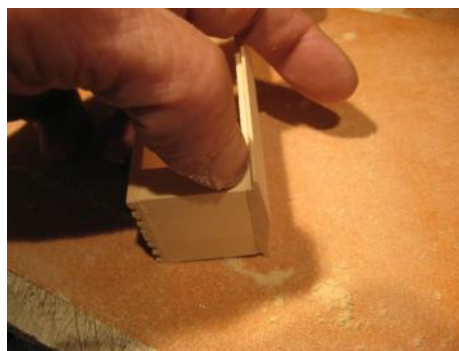
Fig. 16. The fingernail test to ensure edges are sanded even.
