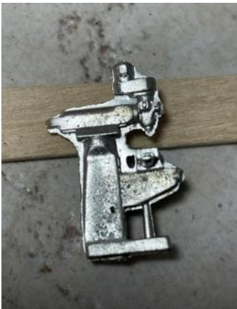
Fig. 2. ASM milling machine before flashing removed.
