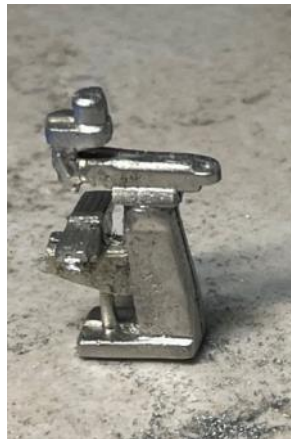
Fig. 3. Milling machine after flashing removed.
