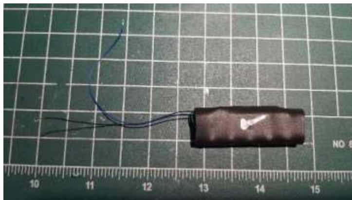
Figure 10 - completed and tested capacitor pack
