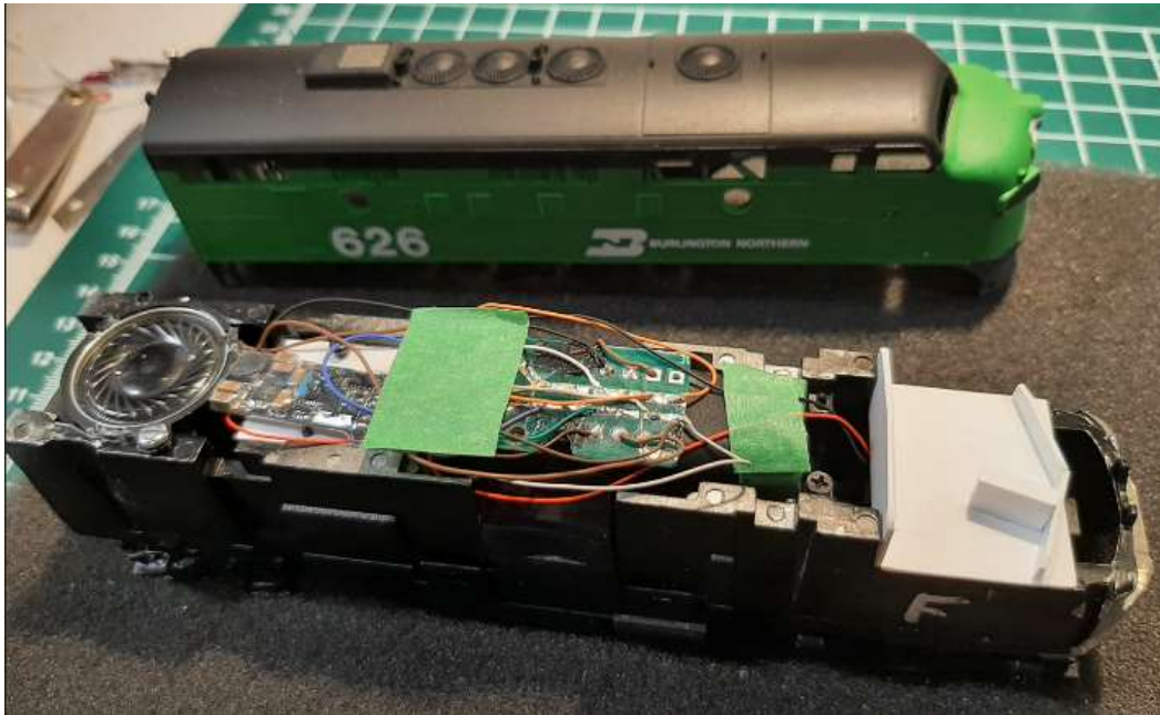
Figure 16 - Proto 1000 F3 mechanism, with capacitor pack, ESU decoder, round speaker, and Inter Mountain F7 shell
