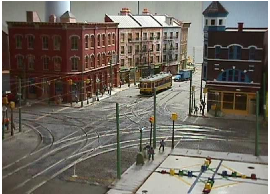
Grand Union—Dual switch and crossover allowing trolleys to move in all directions photo Les Lewis
