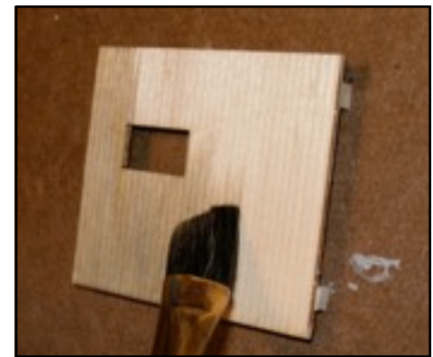
Applying India Ink and Alcohol mix to braced structure wall
